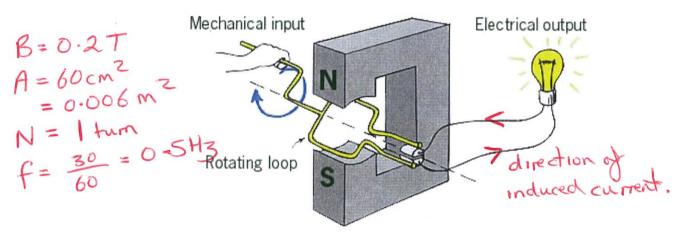
The magnet provides a uniform field of strength 200 mT. The area of the coil of wire is 60 cm<sup>2</sup> and it can be rotated at a rate of 30 rpm.
