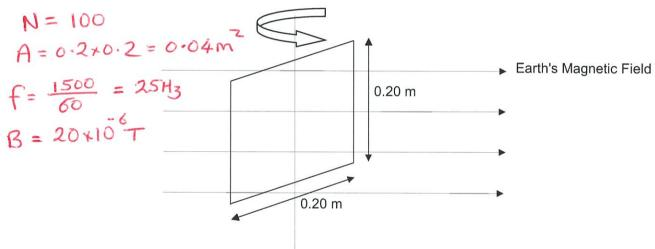
This coil consists of 100 turns of wire and rotates about a vertical axis at 1500 rpm, as indicated in the above diagram. The horizontal component of the earth's magnetic field at this location is  $20 \,\mu\text{T}$ . **Derive** an expression for the **average** voltage induced in the coil by the earth's field and then use it to calculate the **magnitude** of this induced voltage. (5 mar
